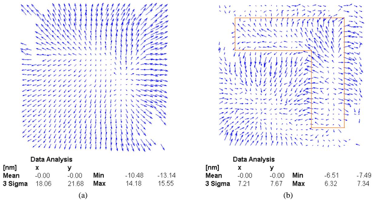
Fig. 5. Experimentally obtained mask distortions due to the etching of a L-shaped pattern in a Cr layer, (a) before and (b) after scale and orthogonality corrections.
