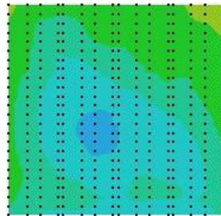
Figure 12: Intra-field wafer CD map after 1<sup>st</sup> CDC treatment
