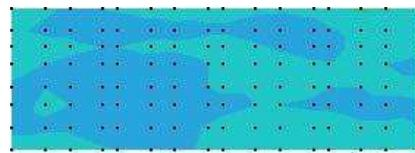
Figure 20: Intra-field wafer CD map after 2<sup>nd</sup> CDC treatment.
