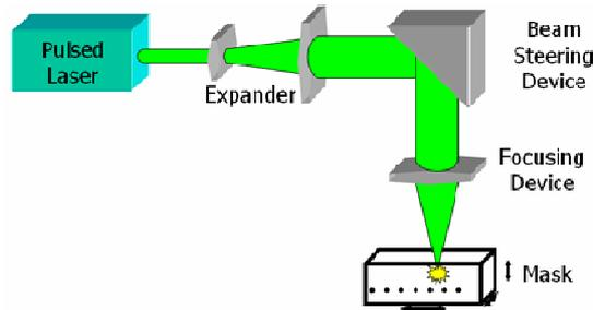
Figure 2: CDC Process: At the focal point of the laser beam a pixel is created. Quartz density is altered, and so is the local index of refraction. Each pixel acts as a scattering element.
