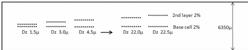
Figure 7: Arrangement of base cells and second layer test cells in the minimum distance between layers experiment.
