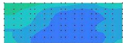
Figure 17: Intra-field wafer CD map after 1st CDC treatment.
