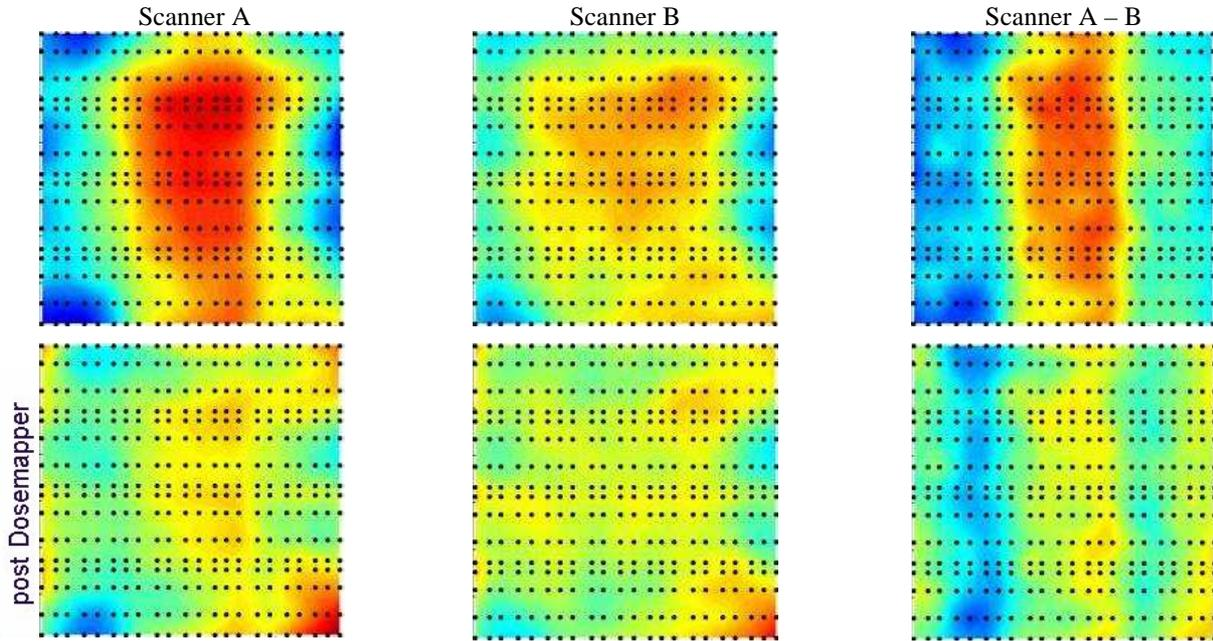
Figure 21: Intra-field CD Map for different scanners
