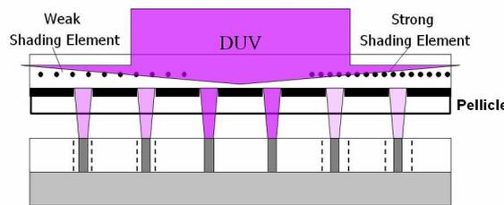
Figure 3: Applying shading elements to the mask reduces light transmission locally and effectively reduces the local dose. This causes all lines to print a CD closer to target.
