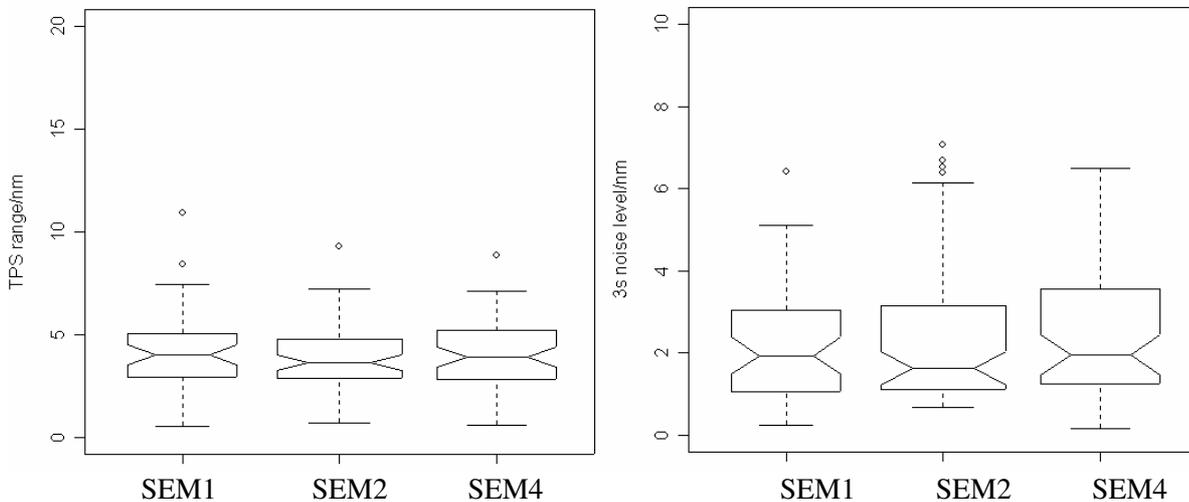
Figure 3: a) Data evaluation from ca. 400 engineering masks mask. An incoherent tool matching exists, since TPS range and 3 sigma noise level shows small deflection. Nevertheless TPS range and noise level are similar, so that the tool matches.
