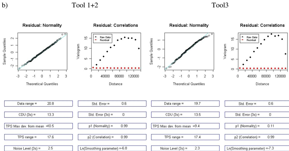
Figure 2: a) CD uniformity plot of a special test mask design with induced CD variations. The test mask was measured on tools from different suppliers and of different technology generations. Since raw data, fit and noise level are almost identical the tools match. b) Data evaluation from mask shown in figure 2a)
