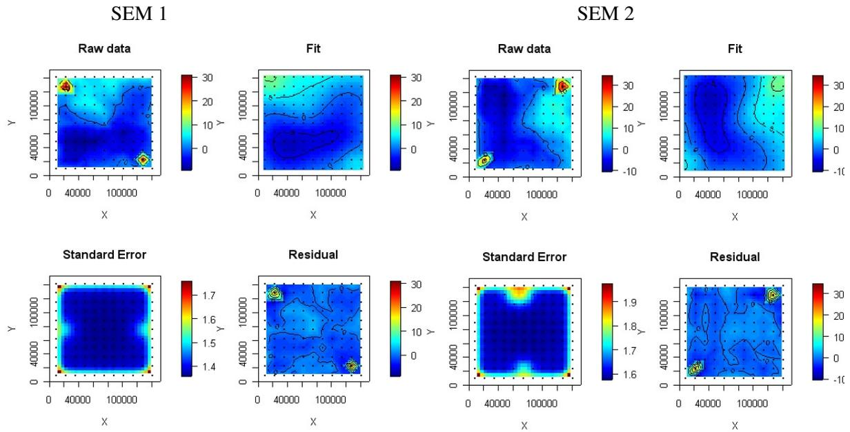
Figure 1: CD uniformity plot of a mask without intentional CD variations. The spatial CD variation over the mask is depicted as a temperature map. Negative CD deviations from the mean are depicted in blue and positive deviations in red. The measurement depicted on the left hand side has been measured at  $0^\circ$  mask orientation, the right hand measurement at  $90^\circ$  mask orientation
