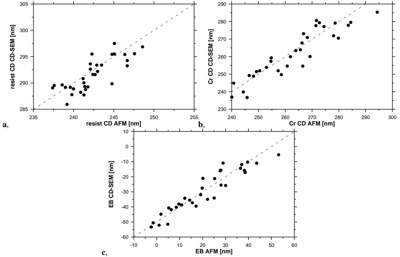
Fig.10 – CD and EB correlations between AFM and CD-SEM measurements. **a**, The resist CD correlation exhibits approx. 50nm difference between CD estimated by means AFM and CD SEM. **b**, Cr CD measurements correlate well with scattering of about  $\pm 5$ nm. **c**, Correlation between the resulting etch biases shows offset of about 50nm.
