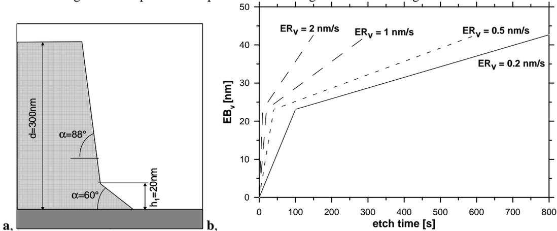
Fig.8 - Transformation of resist side wall shape to vertical etch bias contribution. **a**, represents the side wall slope with resist foot with height  $h_1=20$  nm and slope  $\alpha=60^\circ$ . The slope of the remaining side wall is  $\alpha=88^\circ$  and resist thickness  $d=300$  nm. **b**, shows the vertical etch bias contribution  $EB_V$  according to equation [5] for vertical resist etch rate of 0.2, 0.5, 1 and 2 nm/s. The end of the line corresponds to the 300nm resist thickness.
