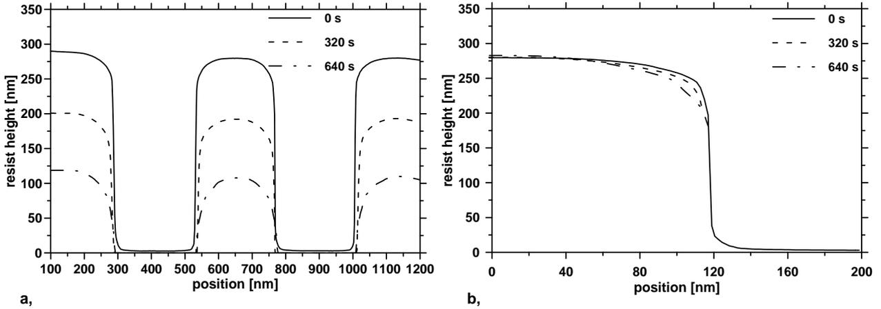
Fig.7 – evolution of the resist side wall. **a**, illustrates the resist side wall shape at beginning of the process, after 320s and 640s. **b**, provides precise comparison of the side wall. The upper approx. 70nm of the resist seems to be etched laterally faster than the remaining side wall.
