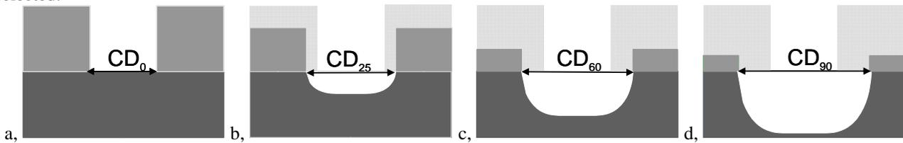
Fig.2 – evolution of the Cr trench during main etch step. Note the widening of the upper edge of the Cr trench at a, 0% b, 25% c, 60% d, 90% endpoint time, described as  $CD_0$ ,  $CD_{25}$ ,  $CD_{60}$  and  $CD_{90}$ .
