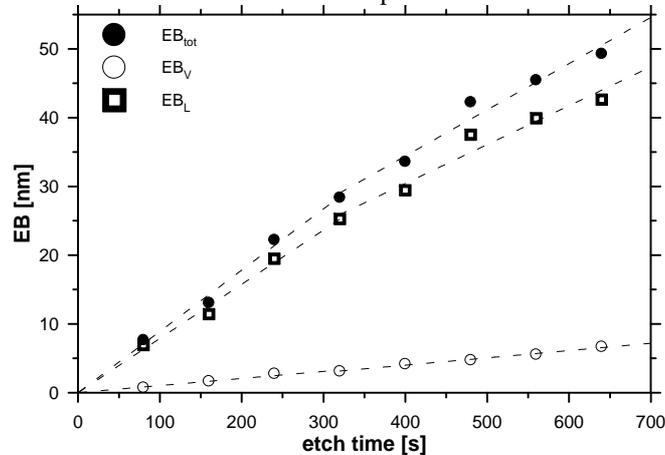
Fig.9 – EB analysis by mean of AFM. The total etch bias  $EB_{tot}$  was identified to contain lateral and vertical EB component as described in text. The vertical component  $EB_V$  is estimated as integral of resist side wall slope and vertical etch rate product process time. Difference between  $EB_{tot}$  and  $EB_V$  component is estimate for the lateral contribution  $EB_L$ .
