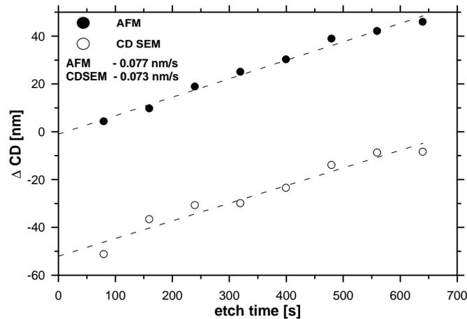
Fig. 5 – comparison of CD evolution as function of time measured at upper Cr edge measured by means of AFM and CD SEM. There is shift in absolute value, however, the slope and so the widening of clear structure is comparable for AFM and CD SEM measurement. The value extrapolated to  $t=0s$  represents the discrepancy between resist CD measured and correct resist CD expected with the Cr CD measurement used.
