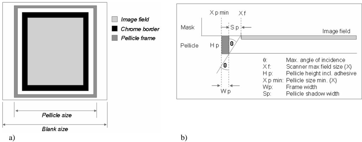
**Fig. 1:** a) Schematic of pelliclized mask (drawings not to scale) b) Pellicle shadow  $S_p$  and minimum pellicle size  $X_{p \text{ min}}$  to avoid shadow and their main influencing parameters (Chrome border not shown)
