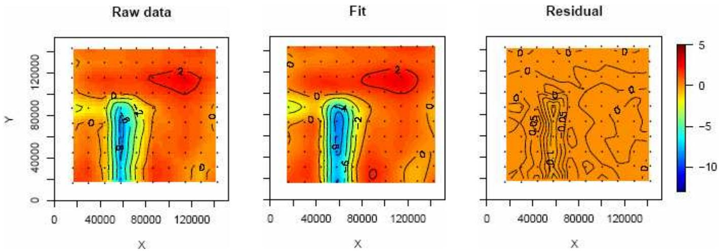
**Figure 2:** *left*) CD obtained using scatterometer for resist measurements, *middle*) TPS fit of the CD data, and *right*) difference plot from CD data and fitted CD data. Scale is in nm.
