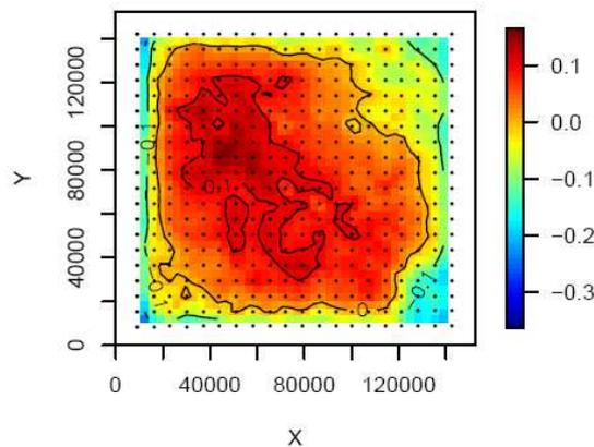
**Figure 3:** MoSi thickness as modelled from the scatterometer data. Scale is in nm.
