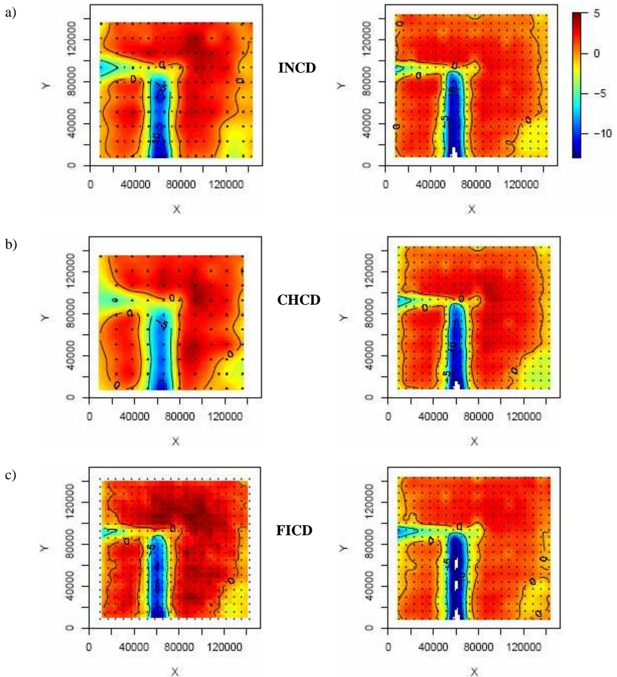
**Figure 1:** CD data obtained by means of CD-SEM (left) and scatterometer (right). 1a) depicts the CD signature at internal CD - Chrome etched, Mosi non etched, 1b) shows the same mask after MoSi etch and, finally, 1c) illustrates the signature after chrome removal. All dimensions are given in nm.
