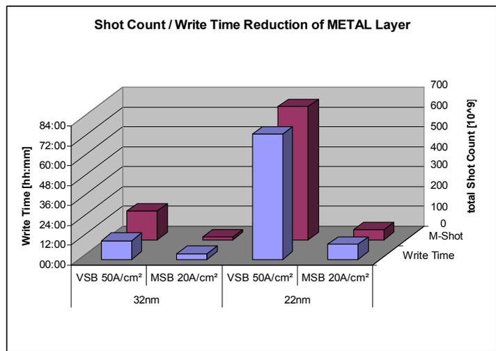
Figure 4: Comparison MSB / VSB advantage 32nm versus 22nm node of Metal 1 layer mask
