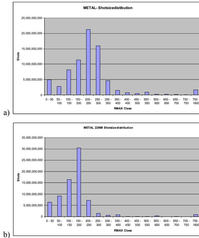
Figure 3: shot size distribution of METAL layers from different technology nodes
