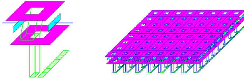
Figure 1: Schematic comparison of single variable shaped beam VSB (left) and Multi Shaped Beam MSB (right) technique
