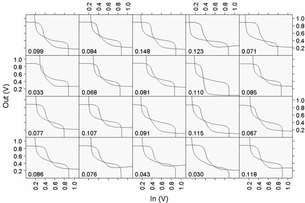
Figure 6 – Butterfly curves for the  $0.076 \mu\text{m}^2$  SRAM flycells in all 20 chips patterned at the contact level with single exposure EUV lithography and at the first interconnect level with double-dipole 193i immersion lithography.
