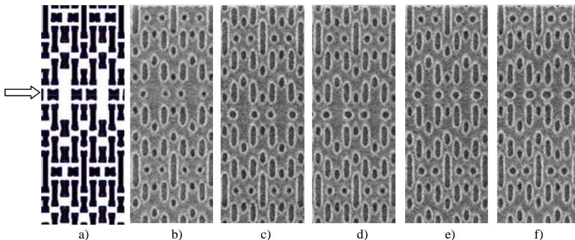
Figure 11 – (a) 80 nm pitch M1 SRAM layout scaled to 56 nm pitch. (b) EUV resist image of 56 nm pitch M1 SRAM pattern corrected for the EUV mask shadow effect but without optical proximity correction. (c)–(f) EUV resist images of 56 nm pitch SRAM pattern corrected for the EUV mask shadow effect and for the optical proximity effect with increasing amount of resist blur.
