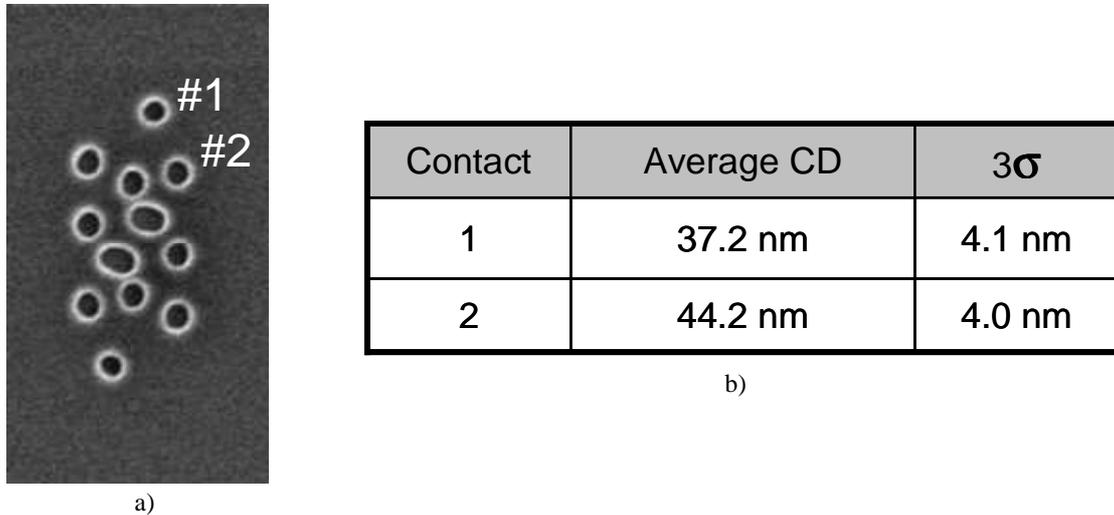
Figure 3 – (a) SEM image of the contact level of a 80-nm pitch SRAM flycell printed in 100 nm thick film of SEVR-78 resist using single exposure EUV lithography. (b) CD control data for contact holes #1 and #2 at 18 mJ/cm<sup>2</sup> dose.
