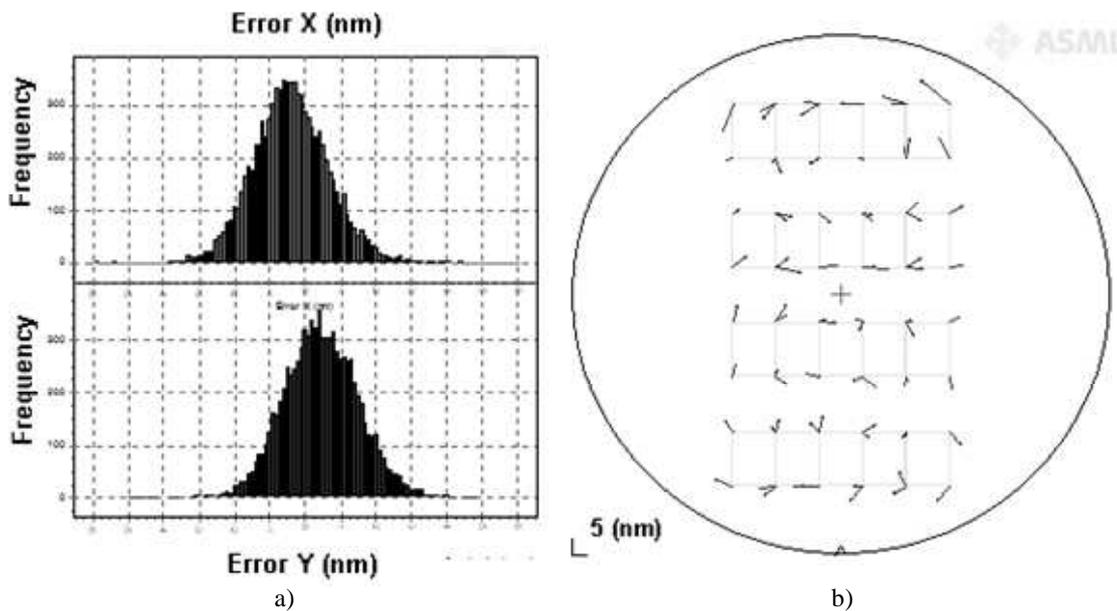
Figure 4 – (a) Single machine overlay data for the EUV Alpha Demo Tool in Albany. The champion, mean + 3 $\sigma$  overlay values were 2.2 nm in x and 2.8 nm in y. (b) Multiple machine overlay data for the contact layer printed with single exposure EUV lithography and the under laying active layer patterned with 193 nm immersion lithography. The mean errors were 1.5 nm in x and 1.7 nm in y and the residual overlay errors were 8.0 nm in x and 7.8 nm in y.
