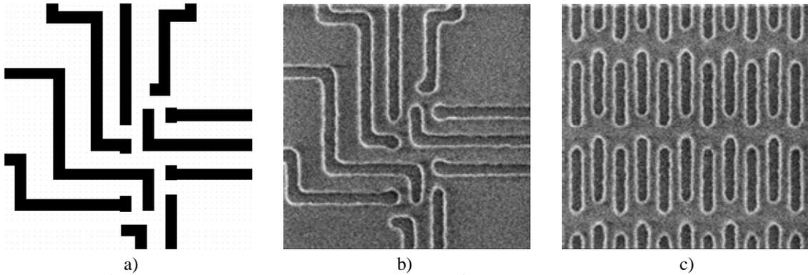
Figure 9 – (a)  $0.08 \mu\text{m}^2$  SRAM flycell layout. (b) EUV images of  $0.08 \mu\text{m}^2$  SRAM flycell in 75 nm thickness of SEVR-139 resist. (c) EUV images of 80 nm pitch first interconnect level dense via chain patterns in 75 nm thick film of SEVR-139 resist.
