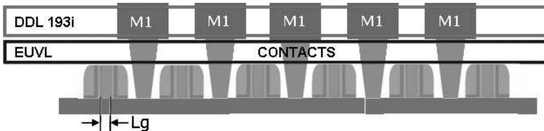
Figure 1 – Integrated stack for 22-nm node test chip in which the contact level was patterned using single exposure EUV lithography and the first interconnect (M1) level was patterned using double-dipole 193 immersion lithography.
