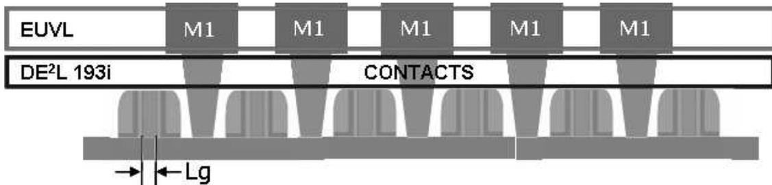
Figure 7 – Integrated stack of 22-nm node test chips in which the contact level was patterned with double-exposure double-etch 193 immersion lithography and the interconnect (M1) level was patterned with single exposure EUV lithography.
