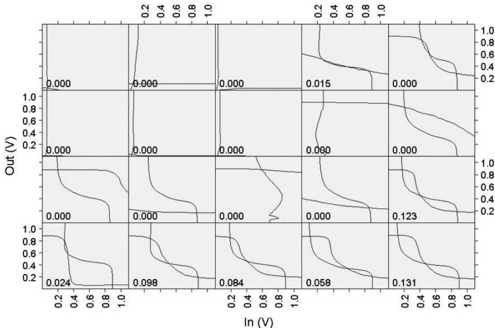
Figure 10 – Butterfly curves for  $0.094 \mu\text{m}^2$  SRAM cells patterned at the contact level with double-exposure double-etch 193 nm immersion lithography and at the first interconnect level with single exposure EUV lithography.
