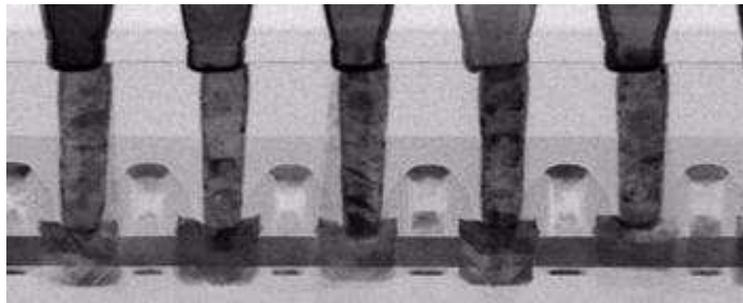
Figure 5 – Cross sectional TEM image of the fully-process  $0.08 \mu\text{m}^2$  6T-SRAM.
