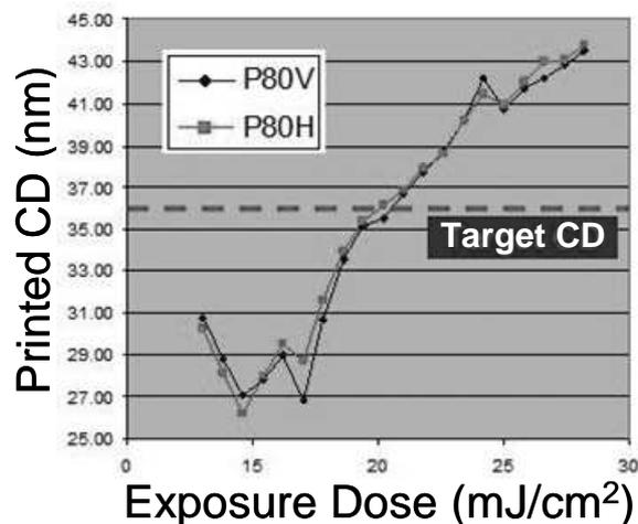
Figure 8 – CD data for imaging of 80-nm pitch line and space patterns in 75 nm thick films of SEVR-139 resist printed with EUV lithography showing that the mask shadow effect correction of the first interconnect level patterns was done nearly perfectly.
