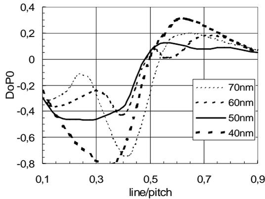
Fig. 11 Degree of polarization (DoP) of the 0<sup>th</sup> diffraction for chromeless Phase shifting masks for different grating structures under optimal dipole illumination as a function of line/pitch.
