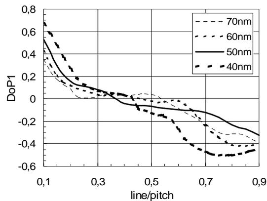
Fig. 12 Degree of polarization (DoP) of the 1<sup>st</sup> diffraction for chromeless Phase shifting masks for different grating structures under optimal dipole illumination as a function of line/pitch.
