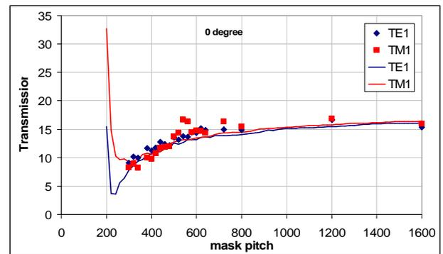
Fig. 6 Normalized transmission of the 1<sup>st</sup> diffraction order of illuminated dense lines /space gratings with fixed duty cycle (line/space=0.5) and varying pitch size under normal incidence illumination: comparison between measurement (squares) and simulation (line).
