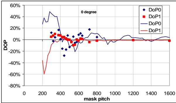
Fig. 7 Degree of polarization (DoP) of 0<sup>th</sup> and 1<sup>st</sup> diffraction orders of illuminated dense lines /space gratings with fixed duty cycle (line/space=0.5) and varying pitch size under normal incidence illumination: comparison between measurement (squares) and simulation (line).
