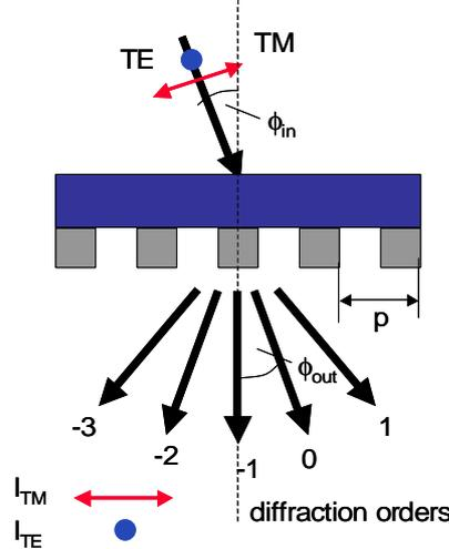
Fig. 1 Schematics of the DoP evaluation set-up
