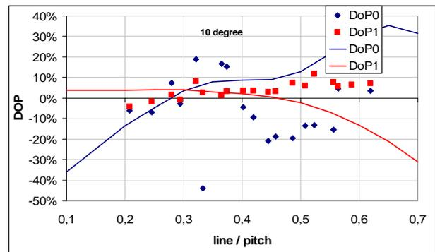
Fig. 9 Degree of polarization (DoP) of 0<sup>th</sup> and 1<sup>st</sup> diffraction orders of illuminated dense lines /space gratings with varying duty cycle and fixed pitch size (400nm) under normal illumination: comparison between measurement (squares) and simulation (line).
