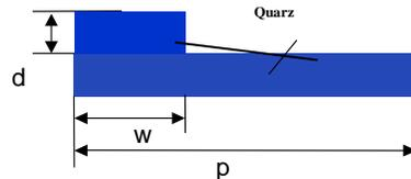
Fig. 3 Structure of unit cell for a chromeless phase lithography mask with  $p$ : pitch,  $d$ : etch depth,  $w$ : line-width
