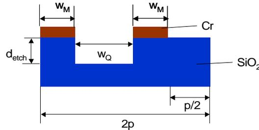
Fig. 2 Structure of unit cell for an AltPSM mask with  $p$ : pitch,  $d$ : etch depth,  $w_M$ : width of chrome absorber,  $w_Q$ : width quartz
