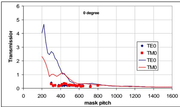
Fig. 5 Normalized transmission of the 0<sup>th</sup> diffraction order of illuminated dense lines /space gratings with fixed duty cycle (line/space=0.5) and varying pitch size under normal incidence illumination: comparison between measurement (squares) and simulation (line).
