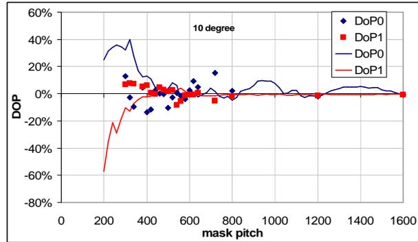
Fig. 8 Degree of polarization (DoP) under 10 degree incidence illumination: comparison between measurement (squares) and simulation (line).
