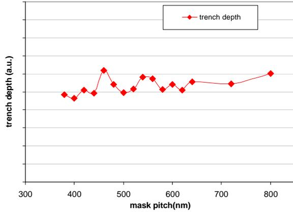
Figure 4 Measured trench depth of Pi-phase-shifting region as a function of the mask pitch.
