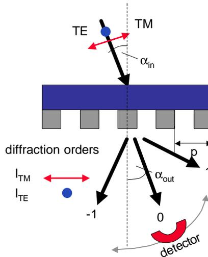
Figure 1 Schematics of the DoP evaluation set-up
