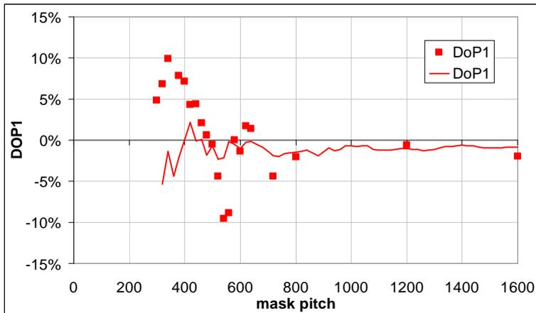
Figure 7 Degree of polarization (DoP) of the 1<sup>st</sup> diffraction order of illuminated dense lines /space gratings with fixed duty cycle (line/pitch=0.5) and varying pitch size under normal incidence illumination: comparison between measurement (squares) and simulation (line).
