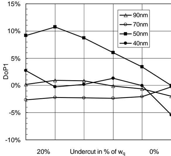
Figure 8 Simulated DoP1 of AltPSM grating structures for different pitches as a function of the undercut size
