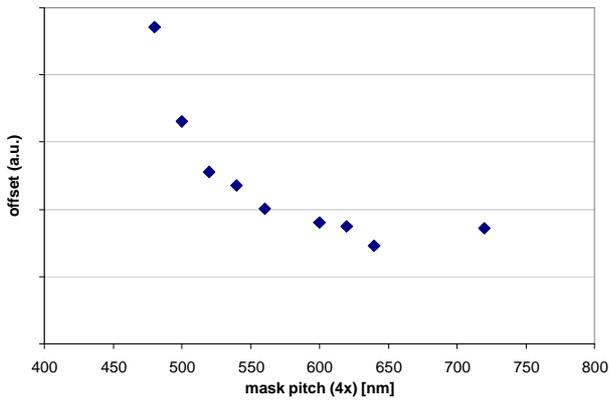
Figure 3 Measured CD offset deviation due to transmission imbalancing of the clear mask structures derived from AIMS measurements.
