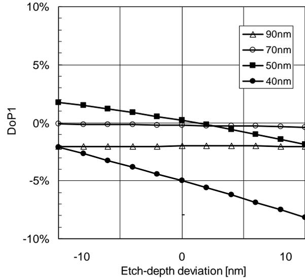
Figure 9 Simulated DoP1 of AltPSM grating structures for different pitches as a function of the deviation of the etch-depth of the ideal Pi-phase shifting etch depth
