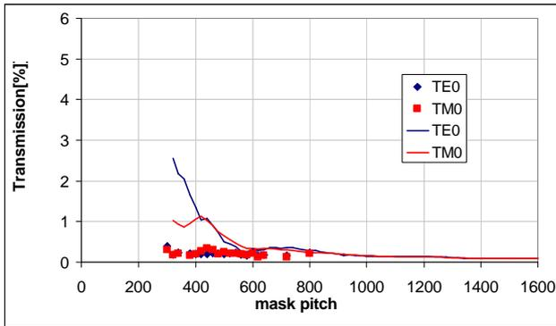
Figure 5 Normalized transmission of the 0<sup>th</sup> diffraction order of illuminated dense lines /space gratings with fixed duty cycle (line/pitch=0.5) and varying pitch size under normal incidence illumination: comparison between measurement (squares) and simulation (line).
