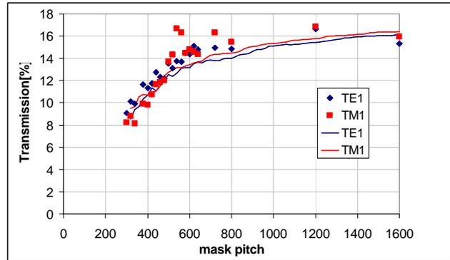
Figure 6 Normalized transmission of the 1<sup>st</sup> diffraction order of illuminated dense lines /space gratings with fixed duty cycle (line/pitch=0.5) and varying pitch size under normal incidence illumination: comparison between measurement (squares) and simulation (line).
