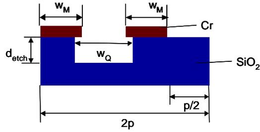
Figure 2 Structure of unit cell for an AltPSM mask with  $p$ : pitch,  $d_{\text{etch}}$ : etch depth,  $w_M$ : width of chrome absorber,  $w_Q$ : width of quartz trench
