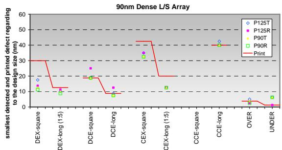
**Fig. 9** Sensitivity analysis for 90nm dense l/s array: Smallest printing and smallest detected defect captured by 100% for four inspection modes (P125 d2dT, P125 d2dR, P90 d2dT and P90 d2dR) is plotted against different types of defects (Fig. 1).
