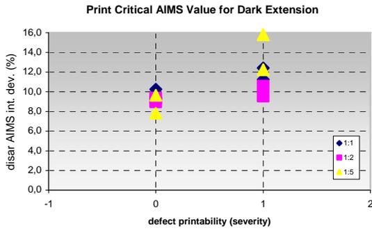
**Fig. 6** Dark extensions: AIMS values for print critical (“1”) and non-critical (“0”) defects at disar exposure and AIMS settings; designed width to length relation of defects is 1:1 or 1:2 or 1:5.
