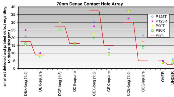
**Fig. 11** Sensitivity analysis for 70nm dense contact hole array (Fig. 2): Smallest printing and smallest detected defect captured by 100% for four inspection modes (P125 d2dT, P125 d2dR, P90 d2dT and P90 d2dR) is plotted against different types of defects.
