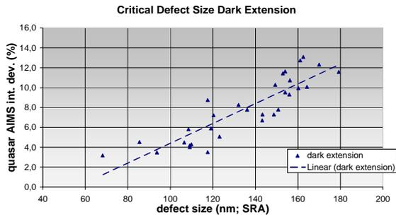
**Fig. 3** AIMS values for dark extension defects received with quasar sigma settings were plotted with respect to defect sizes measured by the SRA method. The chart contain data of “quadratic” and “rectangular” (long) designed dark extensions.
