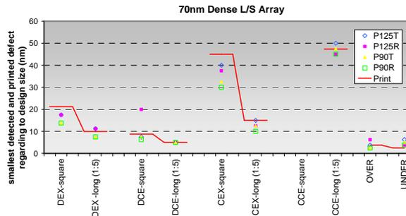
**Fig. 10** Sensitivity analysis for 70nm dense l/s array: Smallest printing and smallest detected defect captured by 100% for four inspection modes (P125 d2dT, P125 d2dR, P90 d2dT and P90 d2dR) is plotted against different types of defects (Fig. 1).
