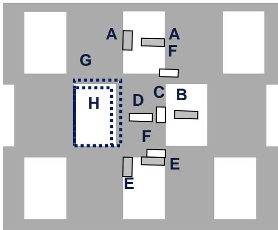
**Fig. 2** Layout for dense 70nm contact hole array with programmed defects. Defect types: A: dark extension (DEX), B: dark center (DCE), C: clear extension (CEX), D: clear center (CCE), E: dark corner (DCO), F: clear corner (CCO), G: over sizing (OVER), H: under sizing (UNDER).
