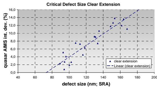
**Fig. 4** AIMS values for clear extension defects received with quasar sigma settings were plotted with respect to defect sizes measured by the SRA method. The chart contained data of “quadratic” and “rectangular” (long) designed clear extensions.
