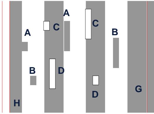
**Fig. 1** Layout for dense 90nm and 70nm 1/s array with programmed defects. Defect types: A: dark extension (DEX), B: dark center (DCE), C: clear extension (CEX), D: clear center (CCE), G: over sizing (OVER), H: under sizing (UNDER).
